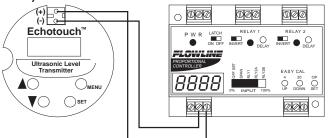
2. Wiring to a Two-Wire Loop Indicator (Model LU20-50\_1):
